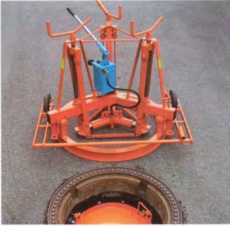
Culvert cover lifter
