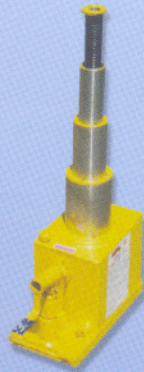
VTEJ-8/425 CAPACITY-8 TONNES LIFT-330 MM CLOSED HEIGHT-210 MM SCREW EXT-95 MM NO. OF STAGES-3
